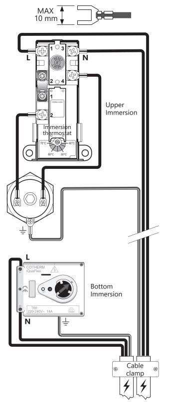
The unit must be connected to a minimum 16 amp dedicated permanent supply complying with current IET Wiring regulations, isolation is required via a minimum 20 amp double pole isolation switch with a minimum 3 mm separation required. All electrical wiring should be carried out by a competent electrician, using a heat resistant cable (minimum 90°C), and be in accordance with the latest IET Wiring Regulations.
